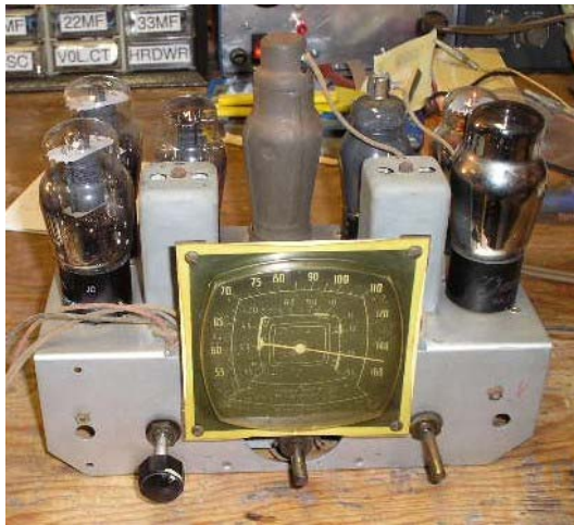
Cleaned, re-capped and aligned chassis
