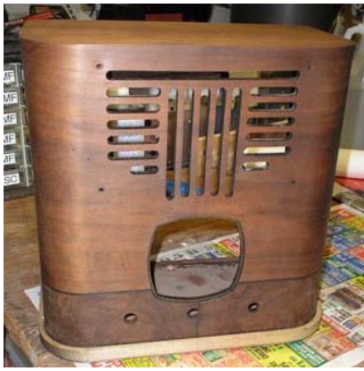
Stripped and cleaned cabinet ready for grain filler
