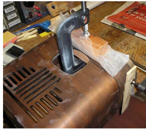
Some loose and split veneer being glued and clamped
